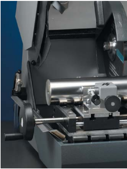
The adjustable cutting table enables parallel sectioning
